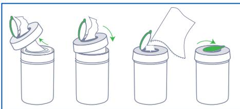
3. Feed the centre wipe through the hole in the cap and replace, Pull wipe at a 45° angle.
