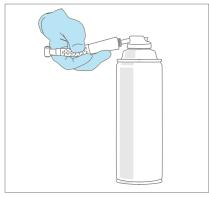
Insert into back of handpiece. Use immediately after each use and before sterilisation. Refer to handpiece maintenance instructions where applicable.
