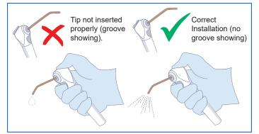
2. CHECK THE TIP IS INSTALLED CORRECTLY
